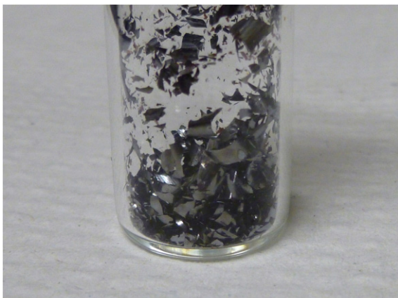
Fig. 4. Picture of a vial containing HWCVD-generated a-Si flakes.
